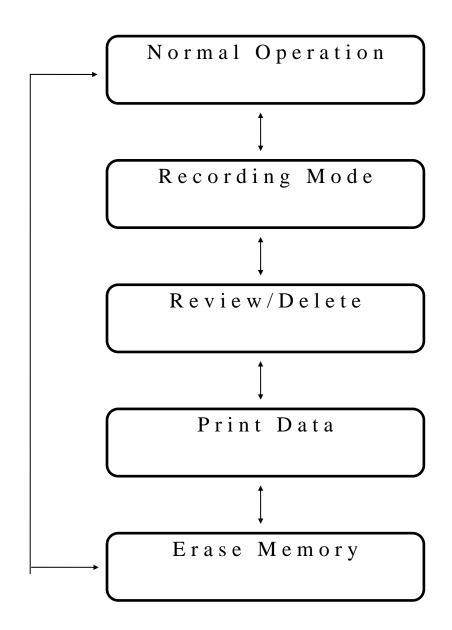
To activate the Memory feature of the YSI Model 52, press the  $\checkmark$  key while the function switch is set to O<sub>2</sub>-TEMP. A display similar to the following will appear:
